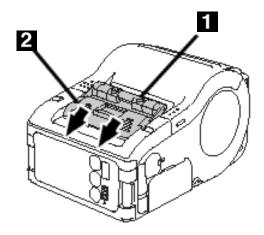
2. Push the black release lever (1) down and toward the front of the printer to open the cover.
